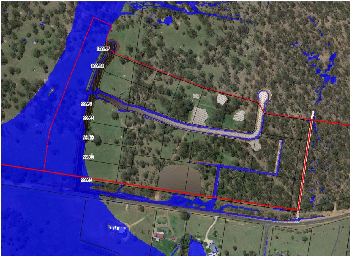
Figure 7.4 – 1% AEP Post-Development Flood Levels
