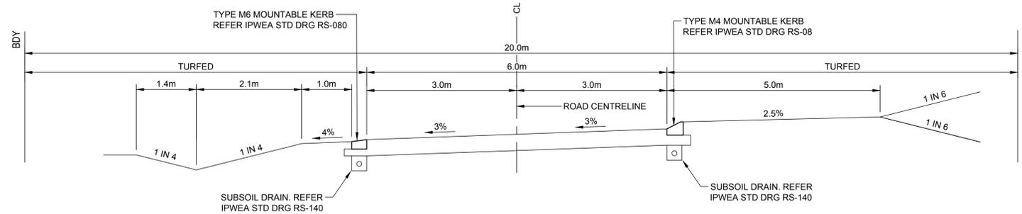
ROAD TYPICAL SECTION - HOWELL CIRCUIT (CH.660 TO CH.785)
