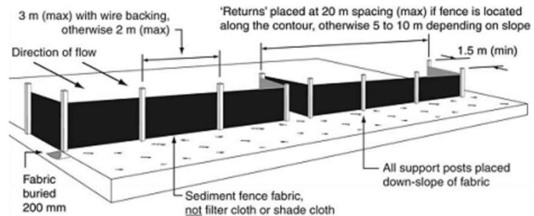
**TYPICAL INSTALLATION OF A SEDIMENT FENCE**
