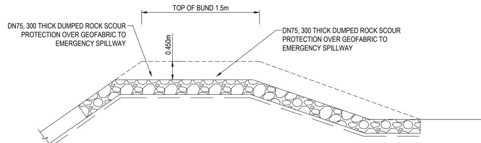
**SEDIMENT BASIN EMERGENCY SPILLWAY DETAIL**
