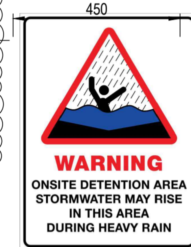
BASIN FLOOD WARNING SIGN DETAIL N.T.S.
