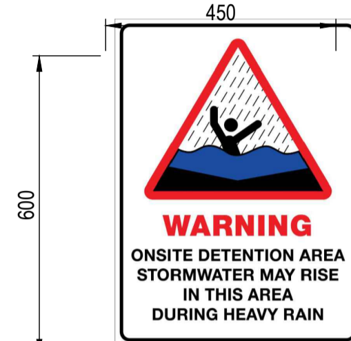
BASIN FLOOD WARNING SIGN DETAIL N.T.S.
